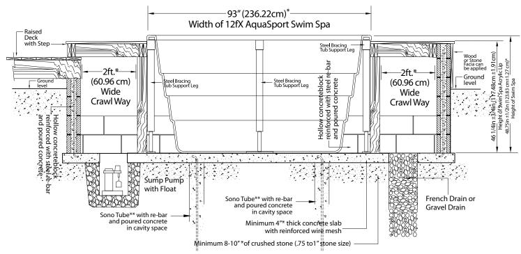
\* Hydropool Inc., can not be held liable for the accuracy of this drawing, its purely provided as a guide only. As each Swim Spa installation has its own set of challenges and variations due to materials used and location of the install. \*\* Sono Tubes only required in installtions that are in regions that experience freezing and thawing.
